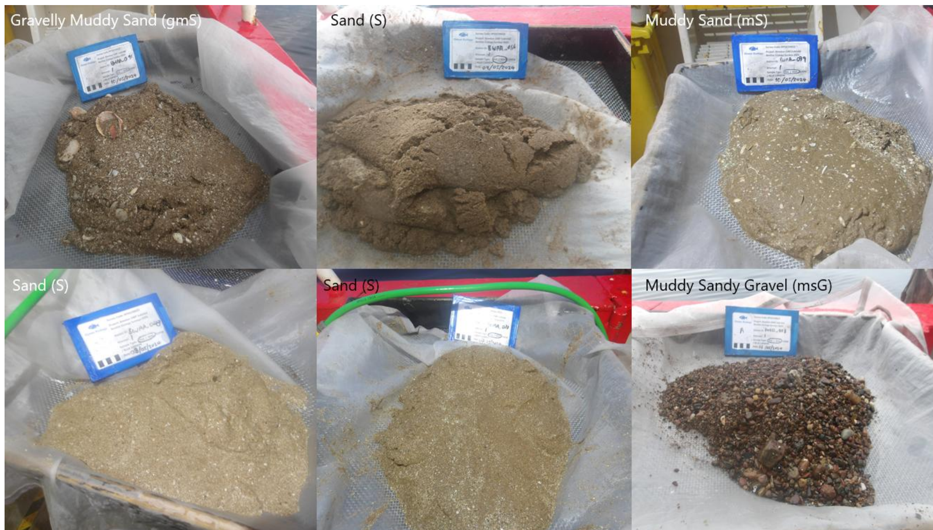
Plate 5 Examples of sediment types found from sieved grab samples. Clockwise from top left: Gravelly Muddy Sand (gmS), Sand (S), Muddy Sand (mS), Muddy Sandy Gravel (msG), Sand (S), Sand (S).
